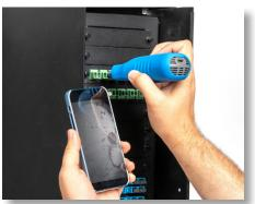
Wireless Fiber Inspection Microscope with APC Adapters.
