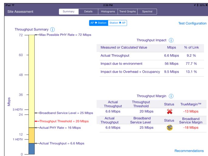
Site assessment analyze throughput and identifies slowdowns
