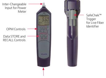
USB Input for Connection to PC for use with VIAVI fiber analysis software
