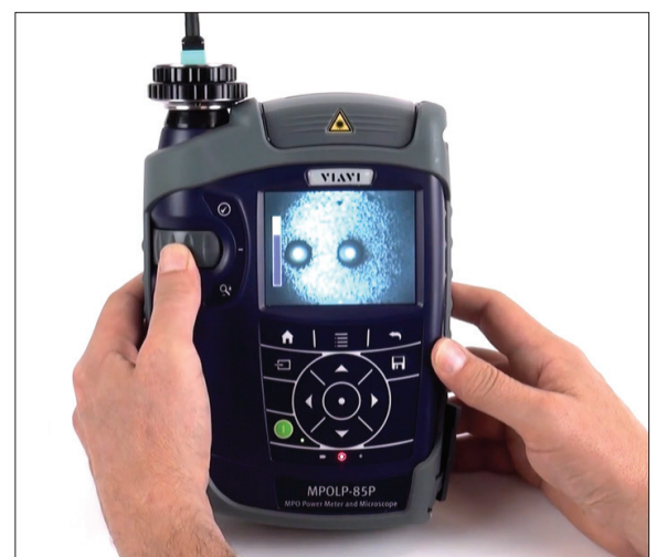
MPO connector inspection with the integrated PCM
