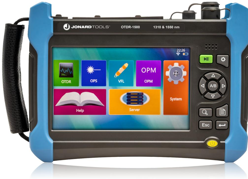
Jonard Tools' Professional Multi-Function OTDR is the perfect all-in-one handheld device for evaluating FTTx and access network construction and maintenance, identifying fiber breakpoints, measuring cable length, and calculating relative optical power losses.
