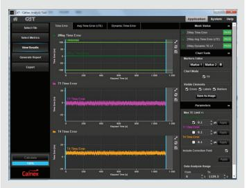
The Calnex Analysis Tool (CAT) provides powerful insight into network and device performance. All your measurement results are now in one place, and you can view multiple graphs simultaneously for easier correlation of your results. Plus, with enhanced graphics, it's easy to evaluate ITU-T metrics such as MTIE, TDEV, MAFE, MATIE against ITU-T masks.
