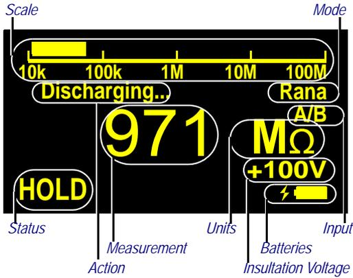
Metro.ISO it is a next generation Insulation Measuring instrument designed and manufactured in Europe with the last technology available in 2014. It can test Insulation-Resistance, Capacitance, AC / DC Voltage, Cable test, Selectable measuring lead pairs.
