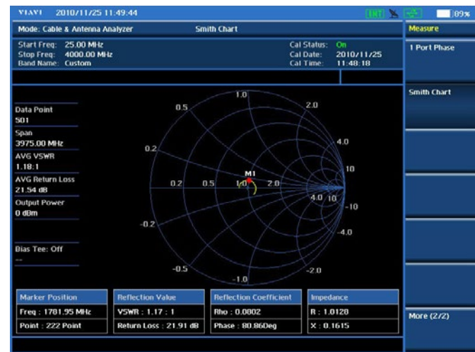
Cable and antenna test — Smith Chart
