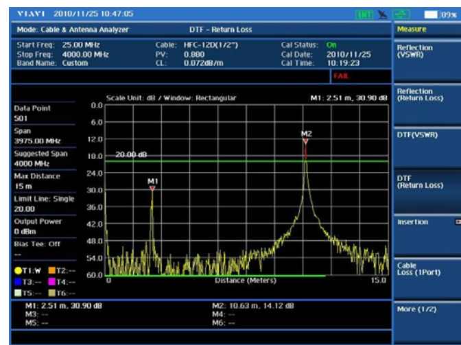
Cable and antenna test — Distance to Fault
