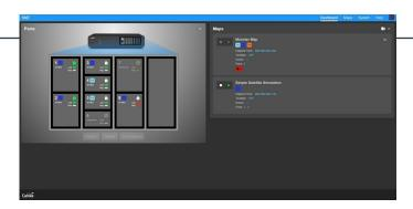
**Ports view** provides information on port configuration, active ports, data rates and link status as well as information on which ports are assigned to which user.
