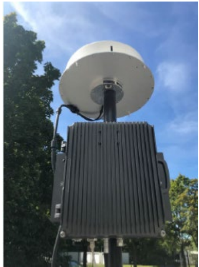
Fig. 1. The SignalShark Outdoor Unit and Automatic DF antenna for AoA and TDOA.
