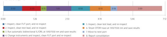
FiberComplete link acceptance procedure:
