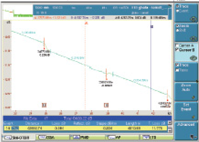
Figure 87. A splice gain on an OTDR trace
