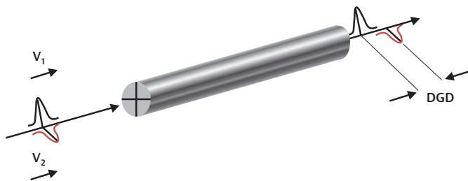
Figure 22. Polarization mode dispersion (or differential group delay) effects on a fiber
