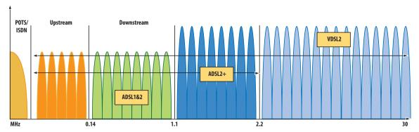
Figure 2. The impact of introducing ADSL 2+ and VDSL2 in copper testing for frequencies up to 30 MHz
